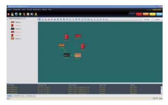
Two-dimensional display of device topology in the home topology interface and alarm association display of communication problems (the color of corresponding alarm icons will also be changed).
