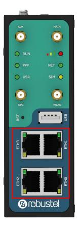
R3000 Quad Router has four Ethernet port with two LED indicators. The yellow one is link indicator and the green one is speed indicator. For details about status, see the table below.
