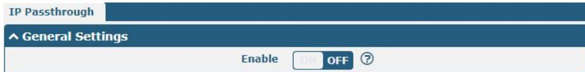
If router enables the IP Pass-through, the terminal device (such as PC) will enable the DHCP Client mode and connect to LAN port of the router; and after the router dial up successfully, the PC will automatically obtain the IP address and DNS server address which assigned by ISP.
