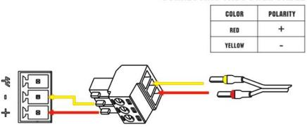
R3000 Lite router supports reverse polarity protection, but always refers to the figure above to connect the power adapter correctly. There are two cables associated with the power adapter. Following to the color of the head, connect the cable marked red to the positive pole through a terminal block, and connect the yellow one to the negative in the same way.
