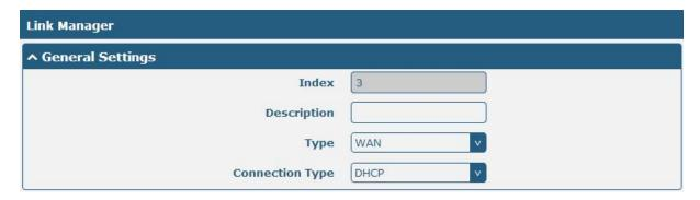
When choose the WAN Connection Type as DHCP, R2000 Dual will obtain IP automatically from DHCP server. When choose the WAN Connection Type as Static.
