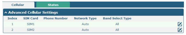
Click to set the SIM card's parameter according to the application requirement.
