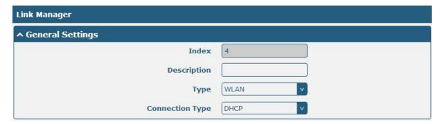
When choose the WLAN Connection Type as DHCP, R2000 Dual will obtain IP automatically from the WLAN AP.
