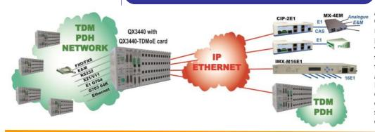
model of the CXR CESoPSN/SAToP/AAL1 range: CIP-2E1, the multiplexer cross-connect QX3440 with **QX3440-TDMoE** card, the IMX-M16E1T1 concentrator of 16 E1 and the IMX-MSTMx concentrator of 32 E1 or 4 STM1/STM4 are compatible together and with equipment from other vendor supporting the same proto-
