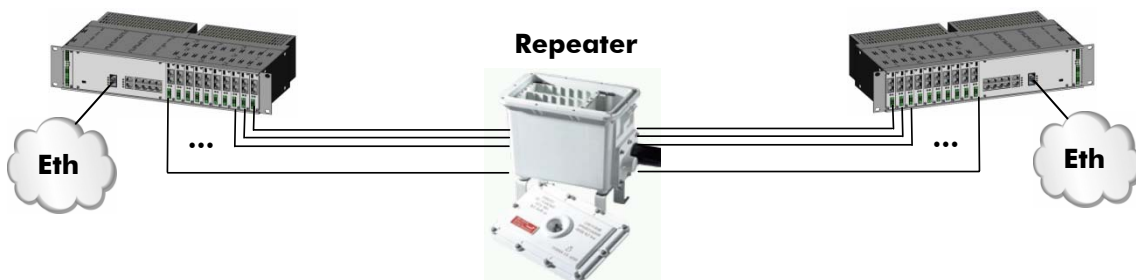
Bonding of up to 20 Copper Pairs, 300Mbps Link
