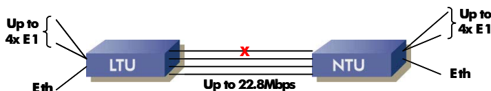
Point-to-Point Bonding Application with Failure Protection
